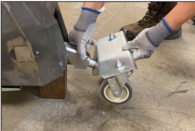
Installing transport wheels.
