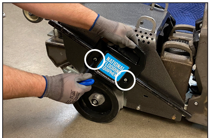
Adjusting slide weight.
