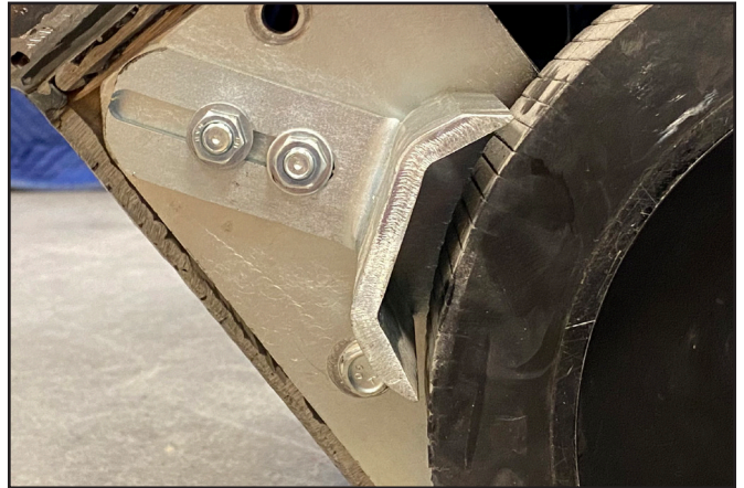
Wheel cleaner adjusted to proper gap.
