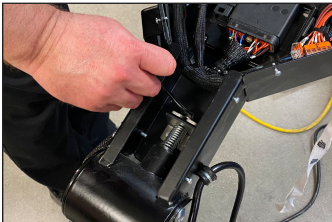
Adjusting the handle release lever.
