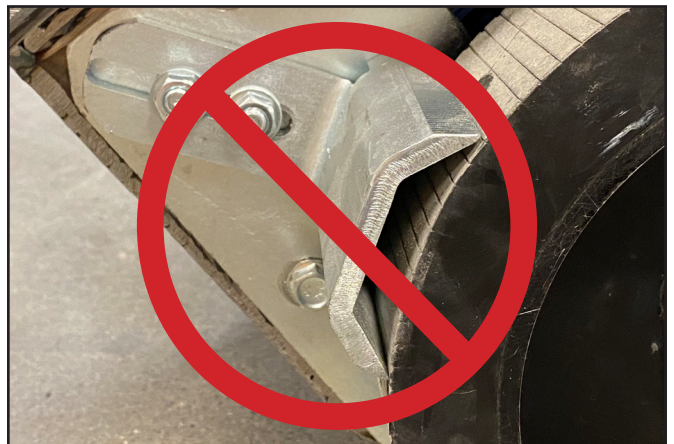
Wheel cleaner should NOT contact wheel.
