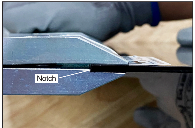
Blade fully seated against notch.
