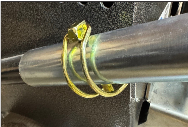
Fig 5 - Locked position of pin.
