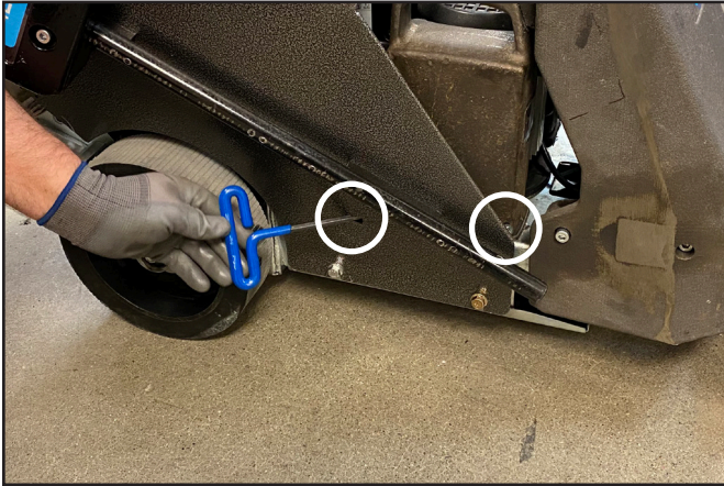
Loosening middle weight locking screws.
